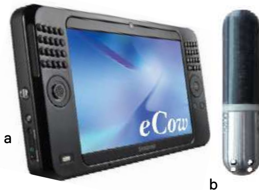
Figure 1 Components of continuous pH measuring device (a) hand-held PC with internal antenna and (b) e-cow bolus.
